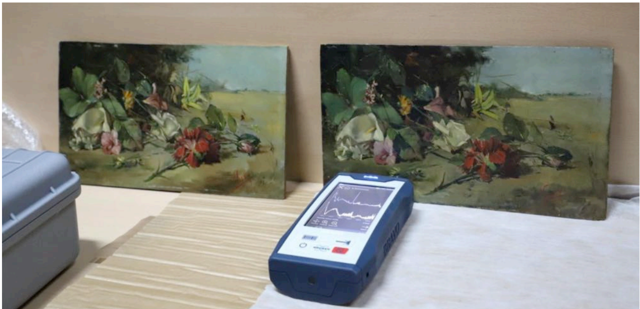
Pigment characterization process in the two works using RAMAN spectroscopy. Source: IVCR+i.
