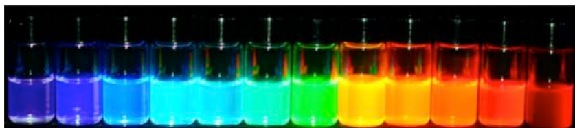
Fig1: Colour tunability of colloidal CsPbX 3 (X= Cl, Br and I) perovskite NCs dispersed in toluene under UV irradiation ( \lambda=365\text{nm} ) [1].
