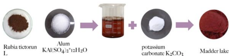
Fig. 1. Recreation of a Madder lake according to the procedure written by Marcucci in the work Saggio analitico chimico. 1816.
